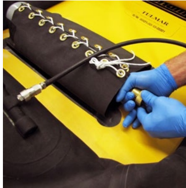
Installing the Air Cylinder
