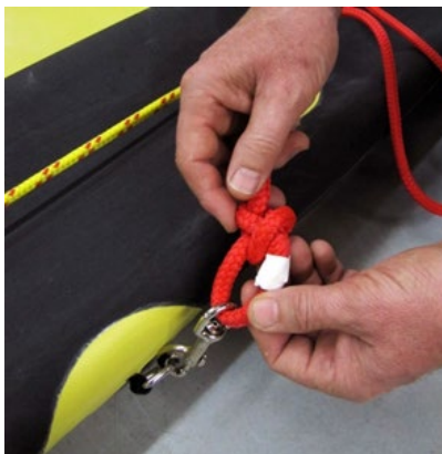
Tape used to Secure Knot on the Pivot Line
