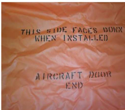
End identifying Aircraft door end And side facing down when installed
