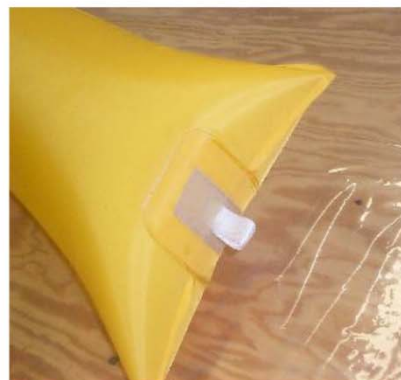
Loop patch on end of Canopy Center and End Support to tie to canopy and slide
