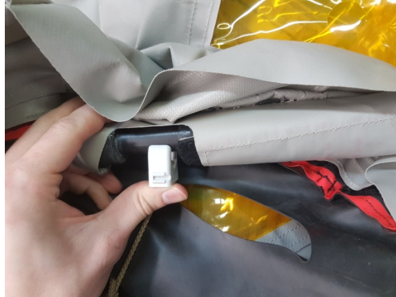
Figure 4: Rearming simulated oxygen cylinder
