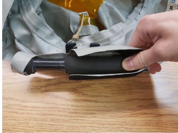
Figure 6: Insertion of simulated O 2 generator
