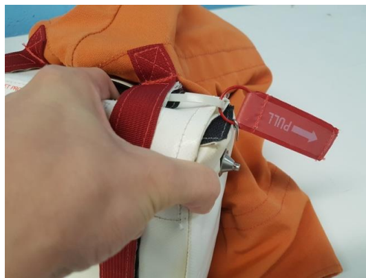
Figure 5: Activation mechanism plunger depressed to reveal hole for actuation pin reset.
