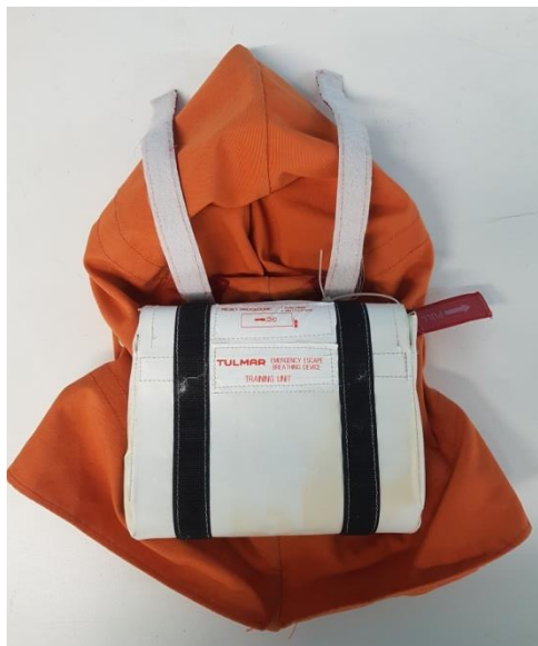
Figure 11: Installing simulated O 2 generator with actuation pin at top right corner
