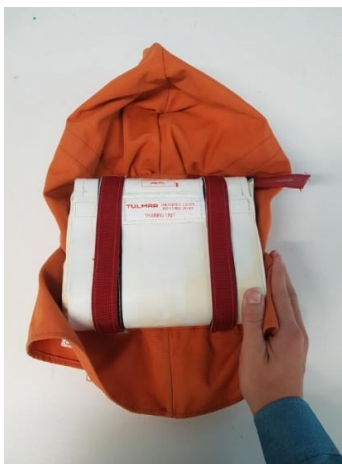
Figure 6: Folding sides of PBE inwards
