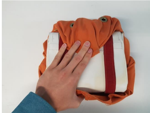
Figure 7: Folding top and bottom of PBE around simulated O 2 generator
