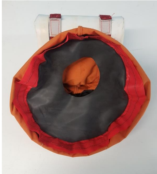
Figure 10: Neck seal orientated with opening closest to rear of hood and Velcro strip facing downwards.
