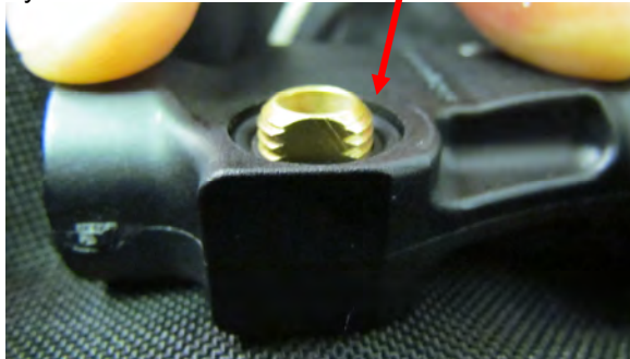
Figure 9: Inflator properly seated on valve stem
