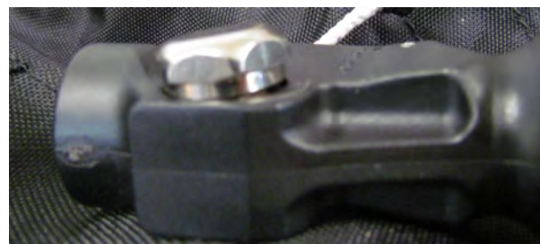
Figure 11: Cross threaded hex cap nut
