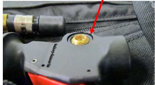
Figure 8: Inflator improperly seated on valve stem
