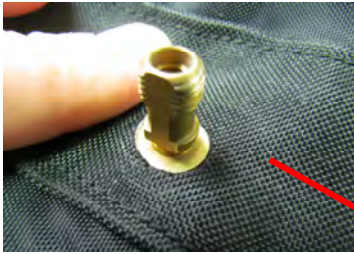
Figure 6: Bladder inflation valve, Ready to install inflator
