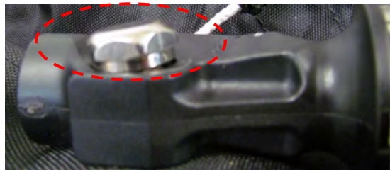
Figure 5: Cross threaded hex cap nut
