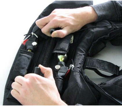
Figure 3.10: Deflation through head lobe deflation valves
