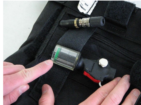
Figure 4.4: Automatic Inflator Cap with Green Indicator
