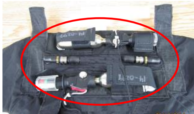
Figure 2 Mechanical inflators to remove
