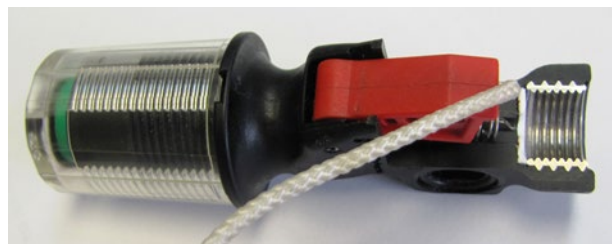
Fig 2.6: Cut-away view of modified Alpha 90000 Inflator with stainless steel insert
