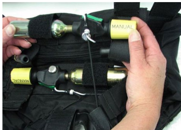
Figure 3.15: Installation of Manual Mode Cap
