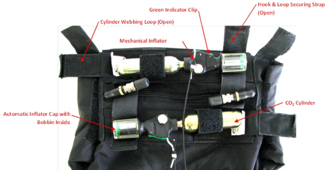
Fig 2.5: Mechanical Inflation System
