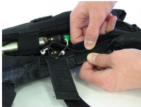
Figure 4.14: Inflation pull cords placed in the pull cord retainers
