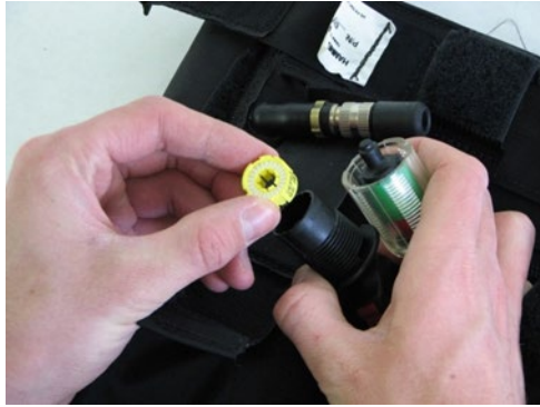
Figure 4.3: Bobbin Replacement
