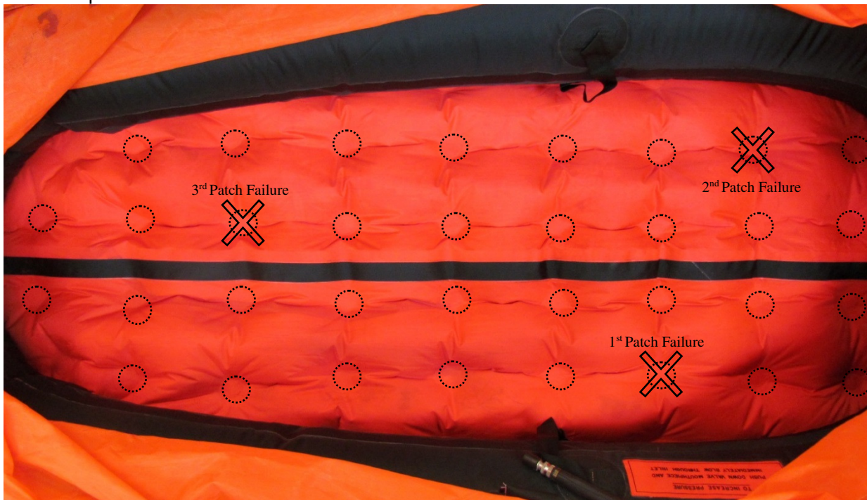
Figure 4: Acceptance criteria 3 – Maximum of 3 patch failures with 2 good patches in between each failure
