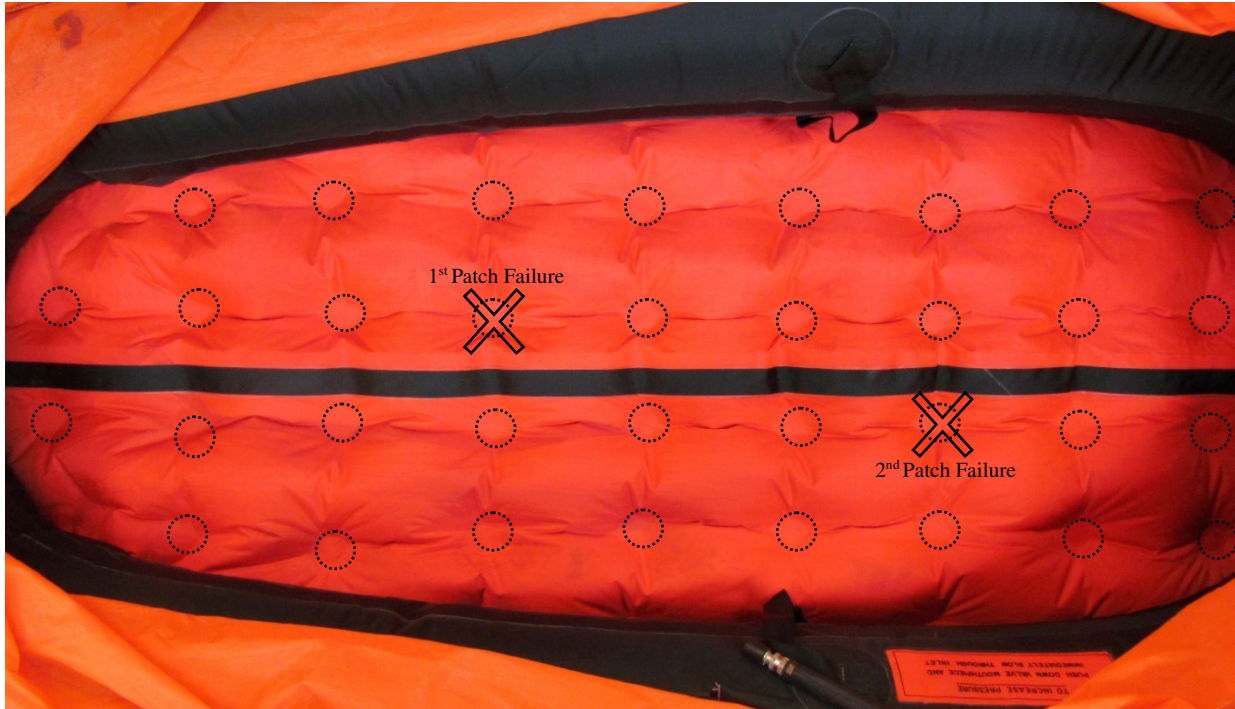
Figure 3: Acceptance criteria 2 – 2 patch failures with 2 good patches in between.
