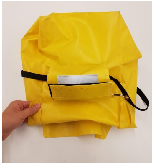
Figure 7: Folding bottom of PBE upwards
