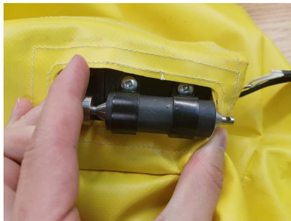
Figure 6: Activation mechanism plunger depressed to reveal hole for actuation pin reset
