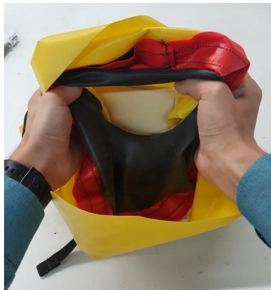
Figure 5: Neck seal stretched open
