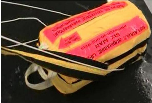
4. As the operating line is pulled further, the CO<sub>2</sub> cylinder operating head is activated and releases the CO<sub>2</sub> gas into the life raft buoyancy chambers.
