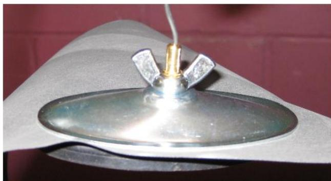
b) Screw stopper into hole as shown by arrow; prepare a patch as soon as possible.
