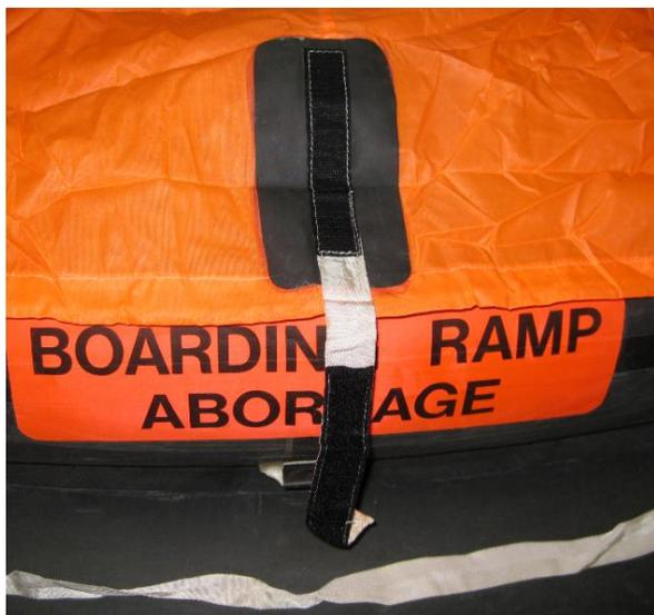
Thread the tape end through the loop on the chamber and back up onto hook portion of Velcro to fasten.
