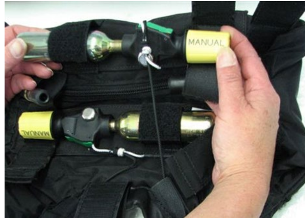
Figure 3.15: Installation of Manual Mode Cap
