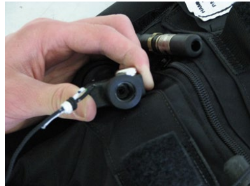
Figure 4.5: Checking Cylinder Gasket at bottom of inflator cavity
