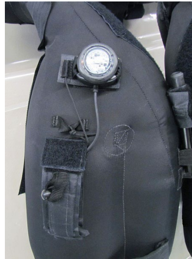
Figure 4.9: Sea light installation
