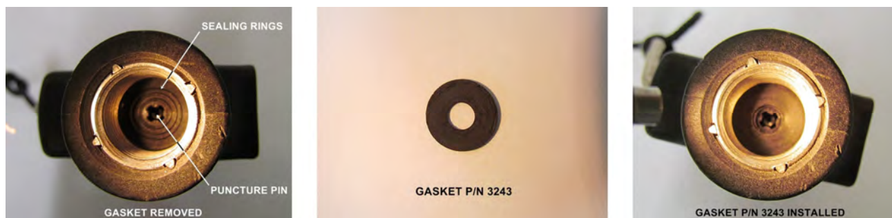
Figure 4, Installing the replacement gasket
