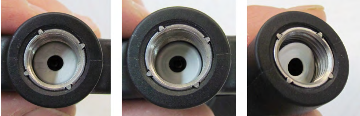
Figure 1, Inflator with white, expanded PTFE gasket
